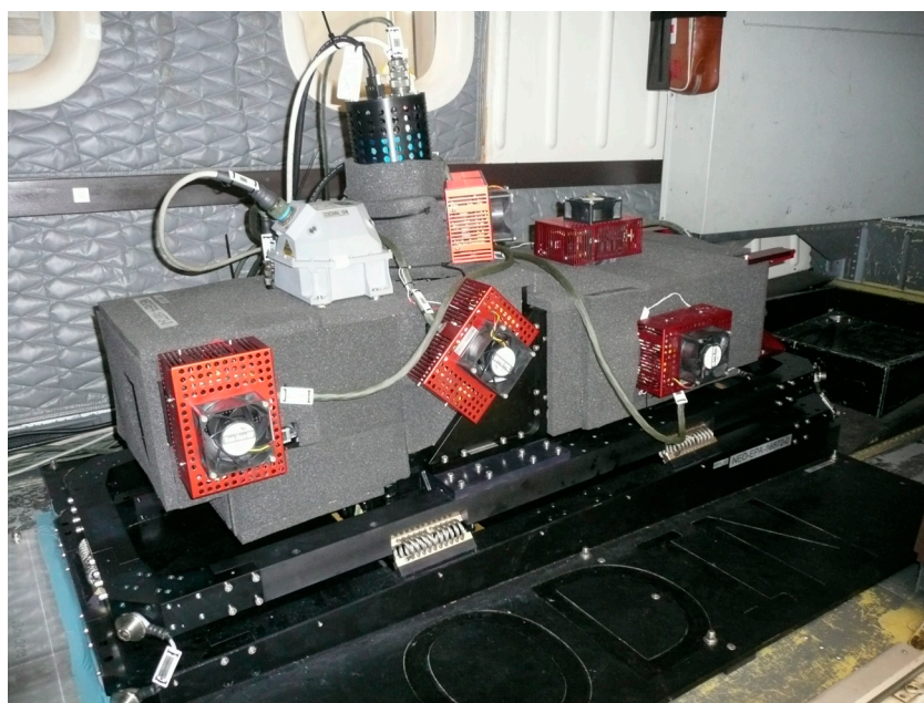
Figure 2: The HySpex ODIN-1024 spectral imager installed into the aircraft.
