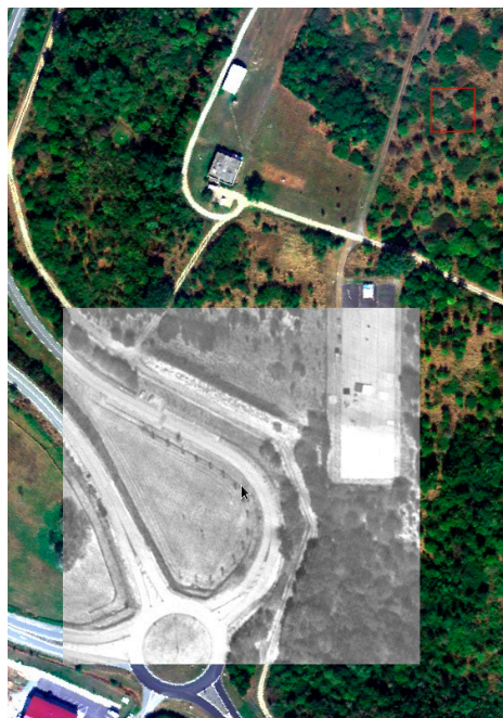
Figure 13: STAD registration result illustration by superimposition of the 4.7 \mu\text{m} spectral band over RGB composition obtained with three spectral bands of the ODIN image
