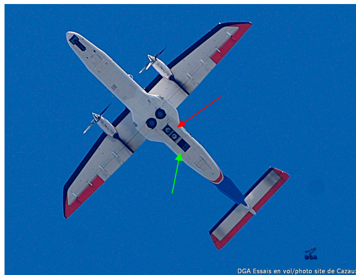
Figure 1: The DO-228 of the DLR with the hatch opened (200 cm \times 50 cm). The two circles (red arrow) are the LWIR and MWIR SIELETTERS components, the black rectangle (green arrow) is the HySpex ODIN instrument.
