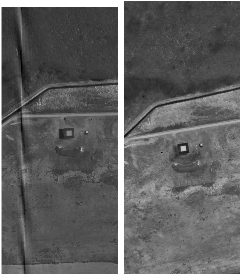
Figure 4, left: MWIR interferometric image from SIELETTERS (note the interference fringes on the left). Right: LWIR panchromatic image for MTF estimation. This image was acquired during another flight in different flight conditions.
