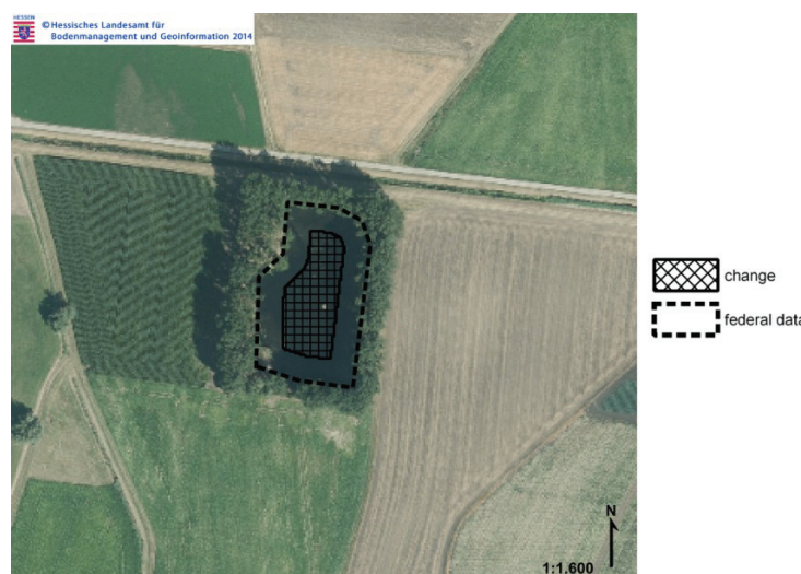
Figure 2: Overshadowed body of water falsely detected as change.
