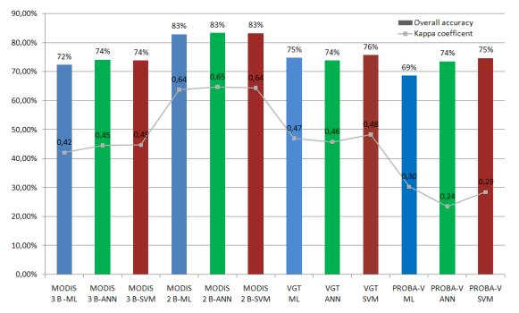
Figure 4: Overall accuracy and Kappa Coefficients or ML, ANN and SVM classification result on MODIS, VGT and PROBA-V (B: bands).
