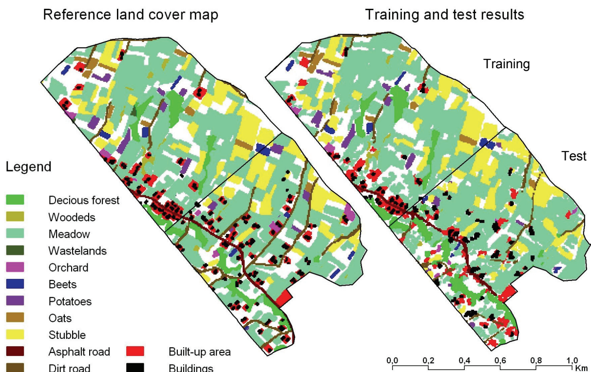
Figure 5: Classification results of the 13 MNF bands (3×3 textural window) of the Biesnik N key polygon.
