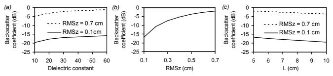
Figure 2: Simulated response of the ERS SAR backscatter coefficient at mid-swath ( $\alpha$  = 23°) to (a) the dielectric constant  $\varepsilon$ , for a smooth (RMSz = 0.1 cm) and medium rough (RMSz = 0.7 cm) surface (L = 5 cm), (b) surface roughness RMSz (L = 5 cm,  $\varepsilon$  = 35) and (c) correlation length L, for a smooth (RMSz = 0.1cm) and medium rough (RMSz = 0.7 cm) surface ( $\varepsilon$  = 35), as predicted by the IEM (11,20).
