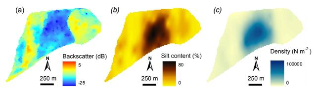
Figure 6: (a) Backscatter derived from a speckle-filtered ESA ERS-1 SAR image, (b) sampled silt content, and (c) sampled total benthic fauna density, Molenplaat, June/July 1995. Outline is the -1.50 m NAP contour line.
