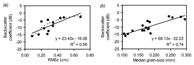
Figure 4: (a) RMSz values (measured perpendicular to the ripple direction) versus the backscatter coefficient estimates derived from an ESA ERS-2 SAR image, Molenplaat, 7 April 2003. The dotted line shows the backscatter as predicted by the IEM for the measured RMSz (with  $\varepsilon$  = 35, L = 5 cm and  $\alpha$  = 21.9°) (b) median grain-size versus backscatter coefficient estimates, Molenplaat, 7 April 2003. The bold lines show linear regression lines, with the regression equations.
