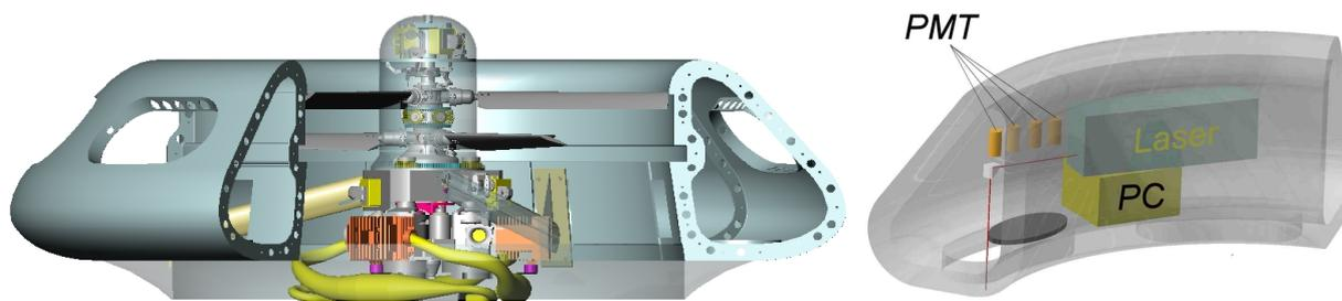
Figure 2: The UAV and its payload. Left: Interior view with rotor hub mechanics and engines; Right: Schematic of the lidar fluorosensor payload with its main components
