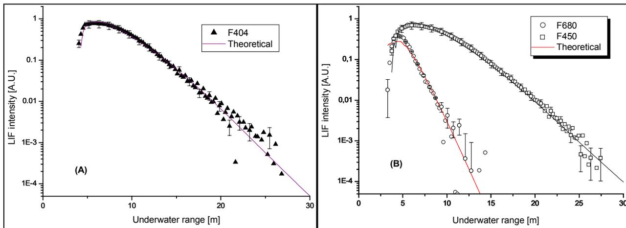
Figure 4: Typical range-resolved LIF signal compared with simulated extinction. Left: 404 nm; Right: 450 nm and 680 nm. [TNB, Dec. 24, 2001].
