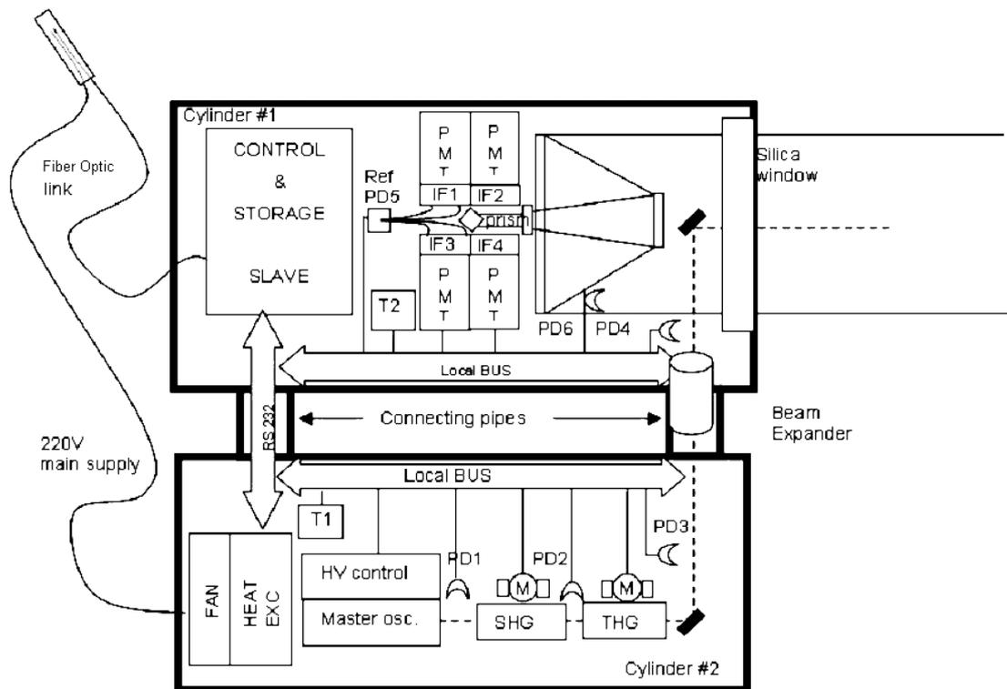
Figure 1: Schematic layout of the lidar payload: PMT (1-4) photomultipliers; IF (1-4) interference filters; PD (1-3) laser emitting photodiodes; PD4 optical trigger photodiode; PD5 emitting reference photodiode; PD6 PAR photodiode; M stepping motor; T trigger signal.
