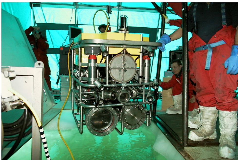
Figure 3: Lidar fluorosensor payload (two cylinders at the bottom of the frame) connected to the ROV, inside the tent during the first Antarctic test (TNB, Dec. 24, 2001).
