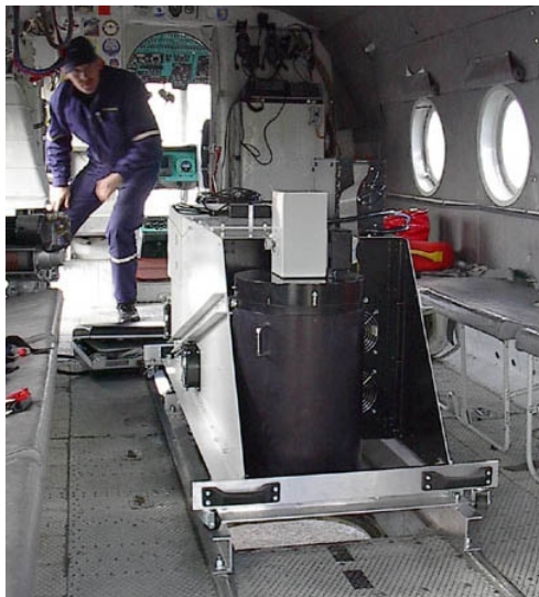
Figure 1: FLS-A lidar installation on board of MI-8 helicopter
