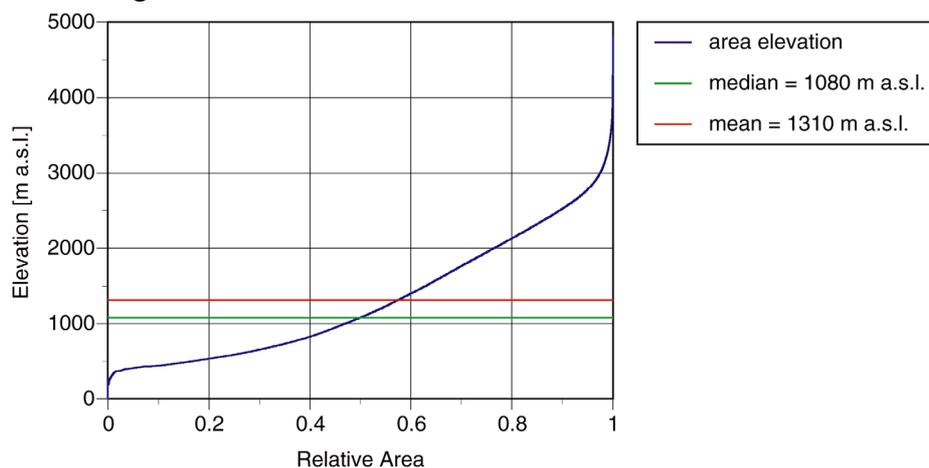
*Figure 1: Area-Elevation for Switzerland (41'242 km)*
