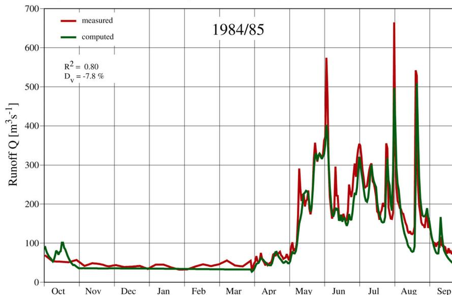
Figure 5: Runoff simulation in Rhine-Felsberg (3,249 km, 562-3,425 m a.s.l.)
