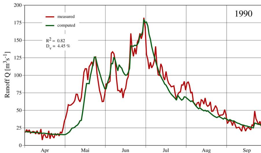
Figure 8: Runoff simulation in Inn-Martina (1,943 km, 1,030-4,049 m a.s.l.)
