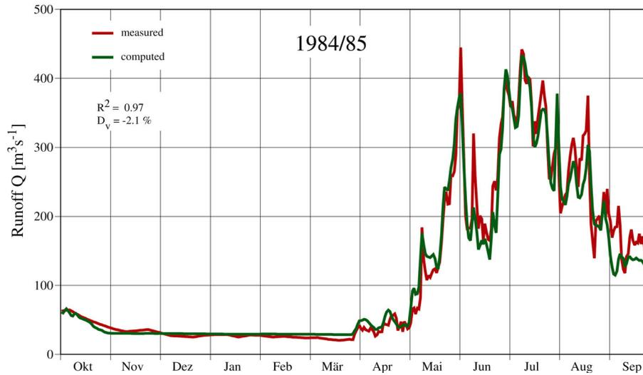
Figure 6: Runoff simulation in Rhône-Sion (3,371 km, 491-4,634 m a.s.l.)
