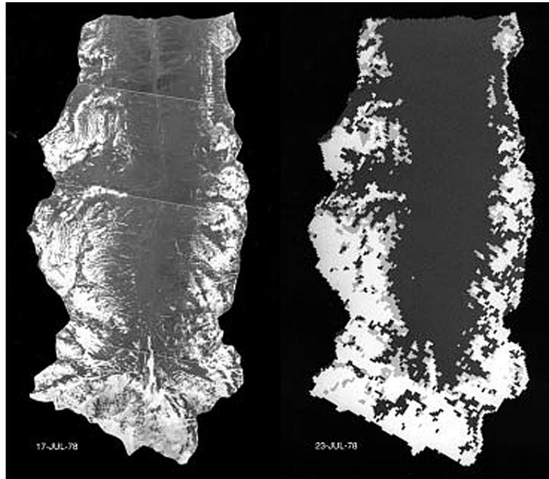
Figure 2: Comparative snow cover mapping in July 1978 in the basin Dischma (43.3 km, 1,668 – 3,146 m a.s.l., Eastern Swiss Alps). Left: Orthophoto, right: Landsat-MSS
