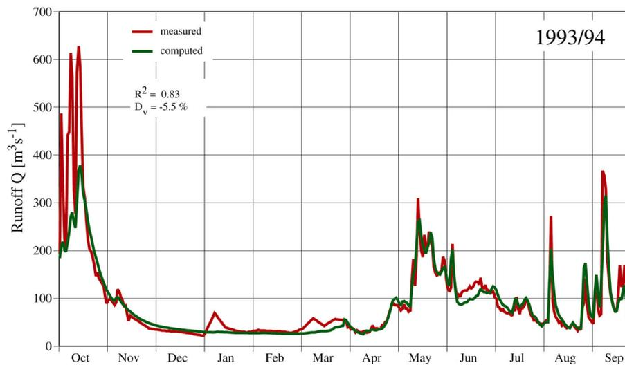
Figure 7: Runoff simulation in Ticino-Bellinzona (1,515 km, 220-3,402 m a.s.l.)
