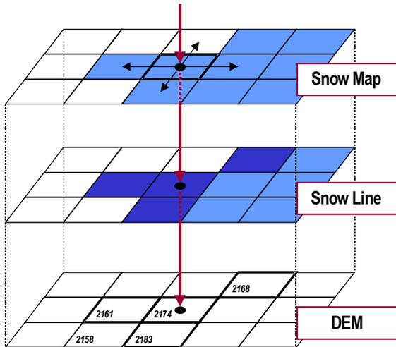
Figure 3: Snow line extraction; based on neighbourhood statistics, snow line pixels are identified and assigned to their corresponding elevation values (DEM: GTOPO30).
