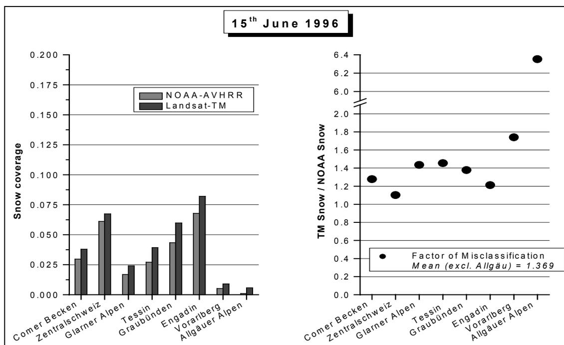
Figure 2: Comparison of snow classification results between NOAA-AVHRR data and Landsat-TM data for one particular day of observation.
