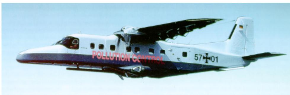
**Figure 1. Maritime surveillance aircraft (Do228LM57+01) operated by the 3<sup>d</sup> Naval Air Wing on behalf of the German Ministry of Transport, Building, and Housing.**
