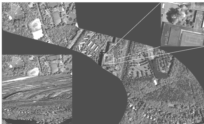
Figure 3. Effectiveness of geometric correction under extreme conditions. Original HRSC-A data (lower left), pre-rectified image data (centre) and enlargement of pre-rectified image (upper right). Flight altitude was 3000 m, ground resolution 15 cm (note that the white lines of a tennis court are quite visible in the enlargement).
