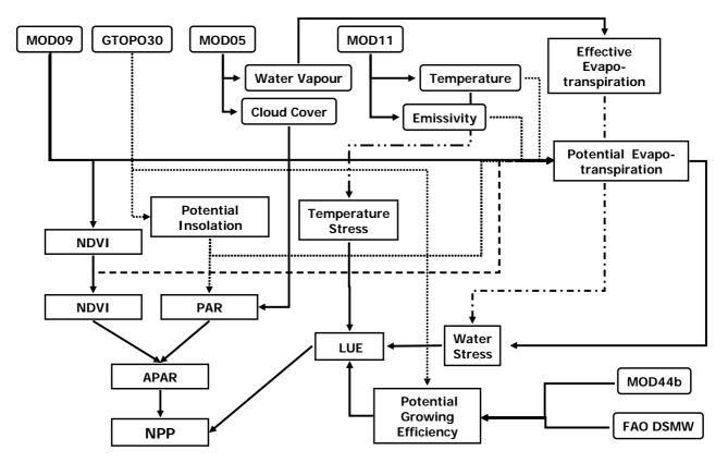
Figure 2: Flowchart of input data for the regional biosphere model RBM. Four MODIS datasets and two auxiliary datasets are integrated into the model.
