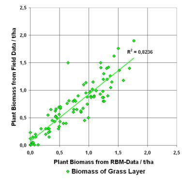
Figure 5: Correlation between grass biomass data from the field and from modelling data. The lower vegetated spots correspond closely to the regression line, while the higher biomass values scatter wider. The variance  $R^2$  of this regression is 82.4%.
